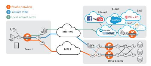
Enhance IT control with SteelCentral Controller: its application-centric, business intent-based policies for path selection enable the solution to derive all path possibilities for applications across the hybrid network. SteelHead products integrate with SteelCentral AppResponse to extend end-user visibility with troubleshooting to SteelHead-optimized and non-optimized, enterprise Web and SaaS applications.
